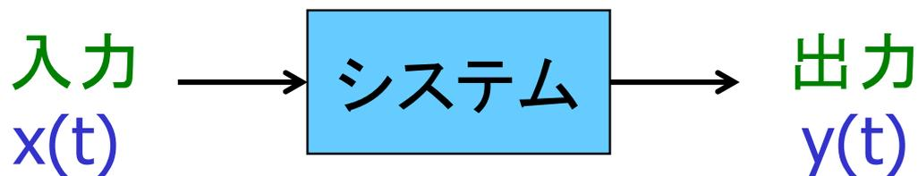
$$b_1 \frac{d}{dt} x(t) + b_0 x(t) = \frac{d^2}{dt^2} y(t) + a_1 \frac{d}{dt} y(t) + a_0 y(t)$$
