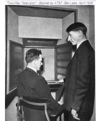
FRANK GRAY and A. L. Johnson in television booth. Behind the glass panels at sides and top are the photo-electric cells.
