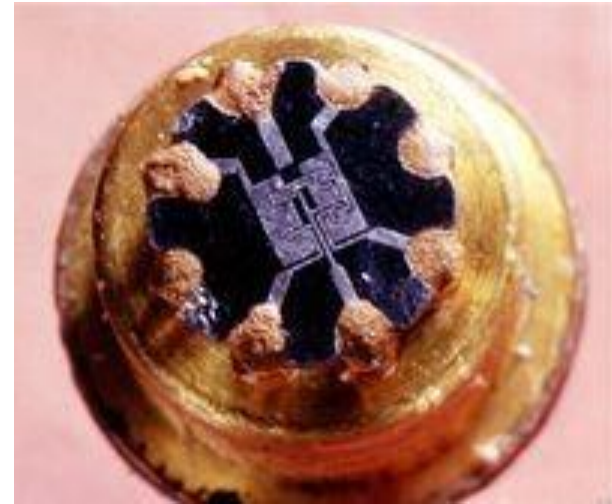
Fairchild Semiconductor Type “F” flip-flop (1960)
