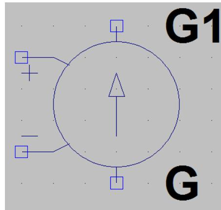
CCVS: Current Controlled Voltage Source
