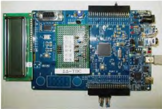
Single-bit \Delta\Sigma TDC with analog FPGA
