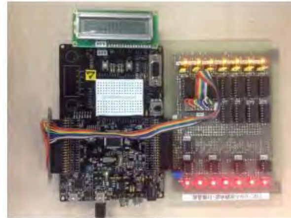
Multi-bit \Delta\Sigma TDC with analog FPGA
