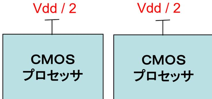
$$\begin{aligned} P2 &= A (V_{dd} / 2)^2 + A (V_{dd} / 2)^2 \\ &= (1 / 2) A V_{dd}^2 \end{aligned}$$
