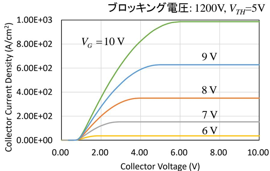
$$W_N = 200 \mu\text{m} \quad p = W_{Cell}/2 = 15 \mu\text{m} \quad L_{CH} = 1.5 \mu\text{m}$$
