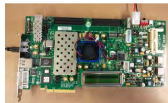
Fig. 12. FPGA board (Xilinx Virtex-6 ML605).
