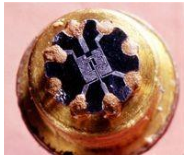
Fairchild Semiconductor Type “F” flip-flop (1960)
