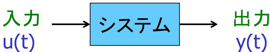
$$\frac{d^n}{dt^n} y(t) + a_{n-1} \frac{d^{n-1}}{dt^{n-1}} y(t) + \dots + a_1 \frac{d}{dt} y(t) + a_0 y(t) = b_m \frac{d^m}{dt^m} u(t) + b_{m-1} \frac{d^{m-1}}{dt^{m-1}} u(t) + \dots + b_1 \frac{d}{dt} u(t) + b_0 u(t)$$
