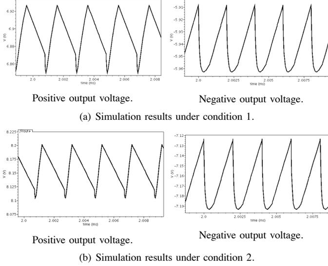
Fig. 3. Transient responses using the conventional timing diagram.
