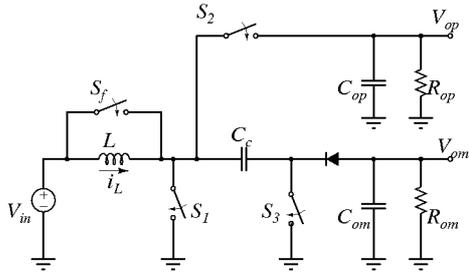
(a) SIMO DC-DC converter schematic [1].
