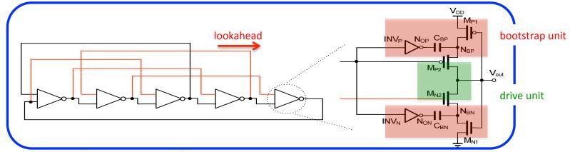
Delay element using bootstrap technique
