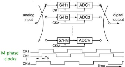
M channel ADCs = M times sampling rate
