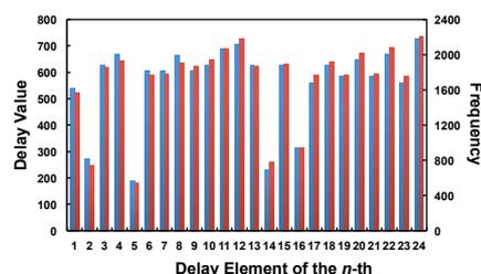
Fig. 2. Histogram and delay values of proposed TDC.
