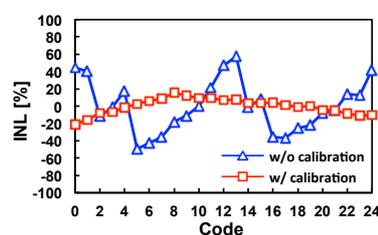
Fig. 5. INL of the TDC with/without calibration.
