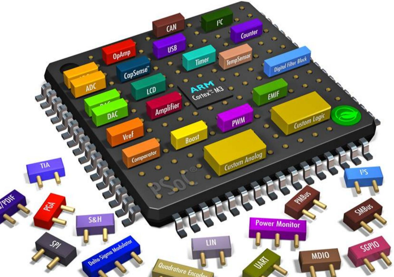
PSoC include a CPU and mixed-signal arrays of configurable integrated analog and digital peripherals.
