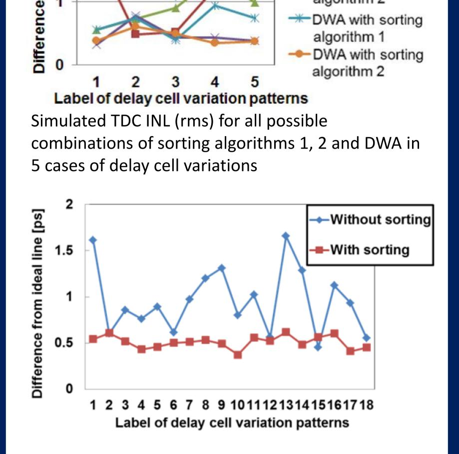
Averaged (rms) integral nonlinearity with and without sorting algorithm 2 in 18 cases of delay cell variations.
