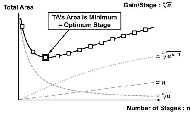
**Fig. 4.** Conceptual image of the design methodology for determining the optimum number of stages.
