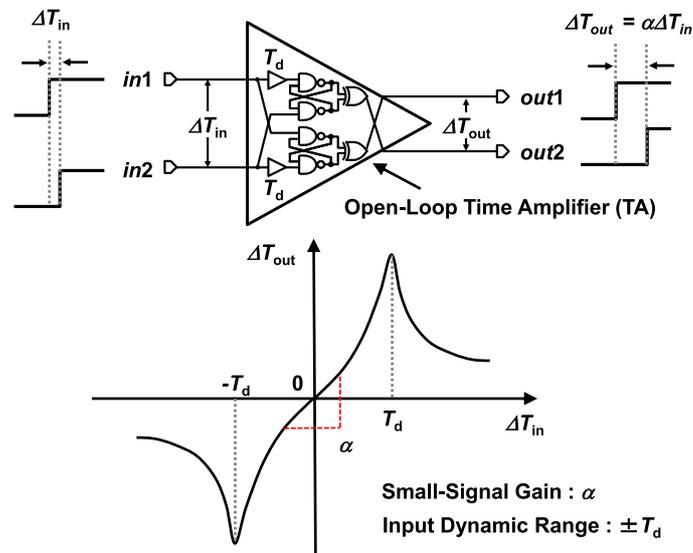
Fig. 1. Schematic of the open-loop time amplifier (TA) [1].
