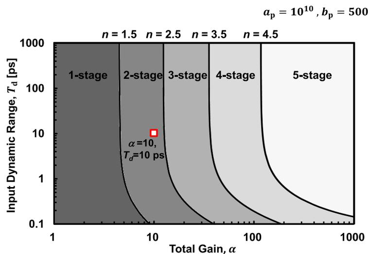
Fig. 6. Design optimization for modification of the specification.
