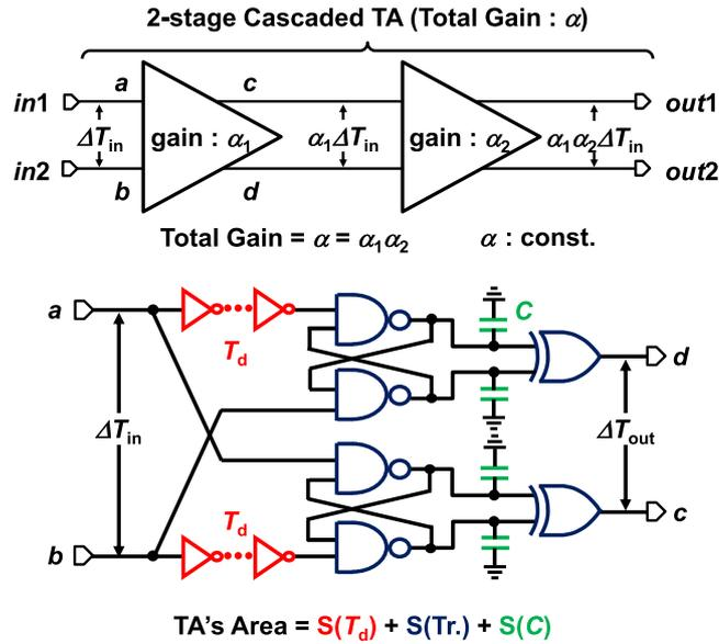
Fig. 2. Schematic of 2-stage cascaded TA.
