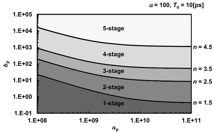
Fig. 5. Design optimization for process porting.
