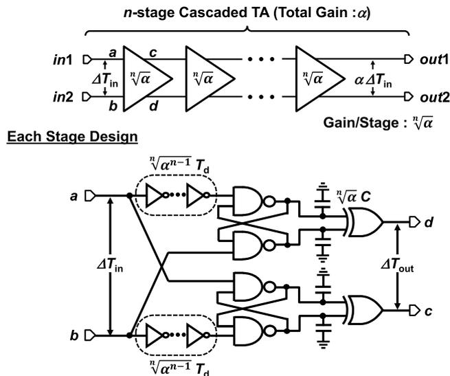
Fig. 3. Schematic of  $n$ -stage cascaded TA.
