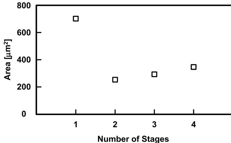
Fig. 7. Occupied area dependence on number of stages.
