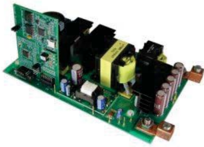
Fig. 4. PSFB DC/DC circuit (Phase Shift Full Bridge DC/DC).
