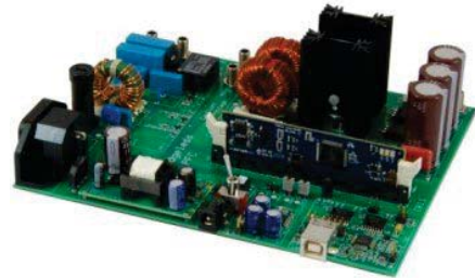
Fig. 3. BLPFC AC/DC circuit (Bridgeless Power Factor Correction AC/DC).
