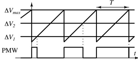
Fig. 3. Relation between  $\Delta V$  and width of PWM signal
