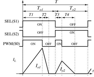
Fig. 5. Waveforms of SEL, PWM signal, and  $I_L$
