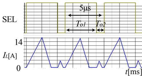
Fig. 15. Waveforms of SEL signal and inductor current in proposed method
