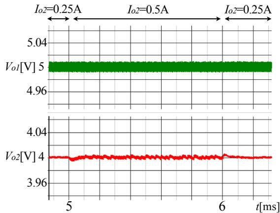
Fig. 19. Load response characteristics when  $I_{o2}$  changed
