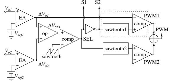
Fig. 8. Block diagram of the proposed control circuit
