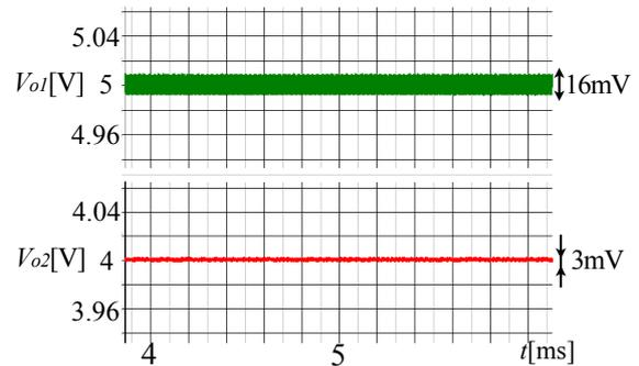
Fig. 17. Steady state output voltage ripple characteristics
