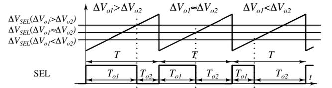
Fig. 9. Relation between the value of  $\Delta V_{o1}$ ,  $\Delta V_{o2}$  and control time ratio( $T_{o1}:T_{o2}$ )
