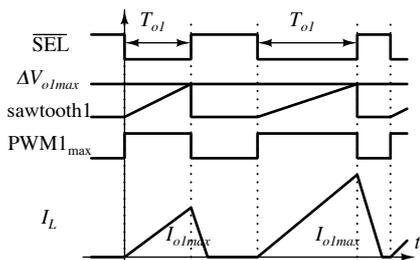
Fig. 13. Increase of PWM signal due to constant peak of sawtooth wave
