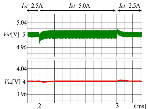
Fig. 18. Load response characteristics when  $I_{o1}$  changed
