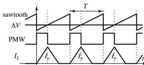
Fig. 2. Waveforms of sawtooth,  $\Delta V$ , PWM signal,  $I_L$
