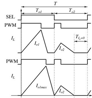
Fig. 6. Maximum value of  $I_{o1}$  in conventional method
