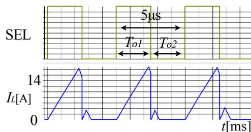
Fig. 14. Waveforms of SEL signal and inductor current in conventional method
