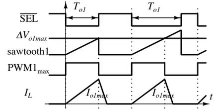
Fig. 11. The relation between peak value of sawtooth wave and maximum width of PWM signal
