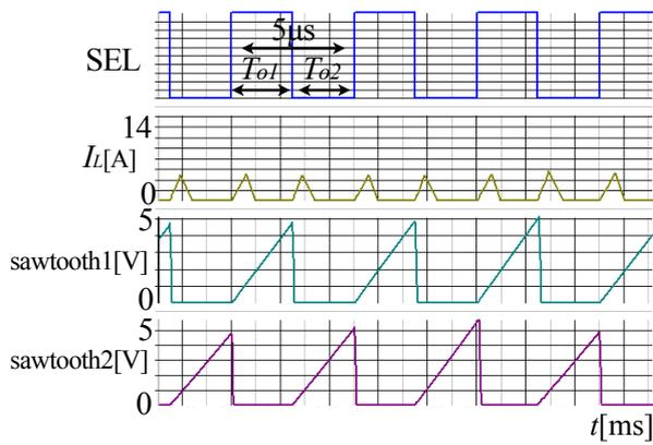
Fig. 20. Waveforms of SEL,  $I_L$ , sawtooth1 ( $I_{o1}:I_{o2}=0.5A:0.5A$ )
