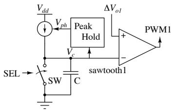
Fig. 12. The sawtooth wave generator circuit with variable pulse width
