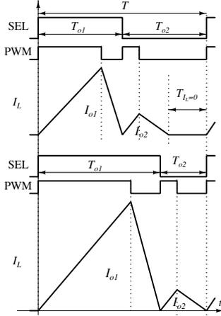
Fig. 7. Change of  $I_{o1max}$  by increasing  $T_{o1}$
