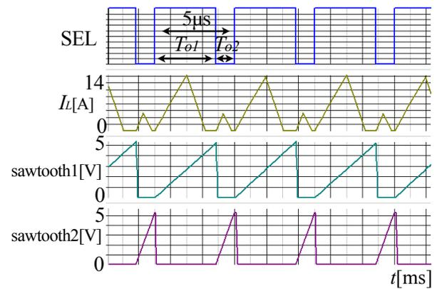
Fig. 21. Waveforms of SEL,  $I_L$ , sawtooth1 ( $I_{o1}:I_{o2}=5.0A:0.5A$ )
