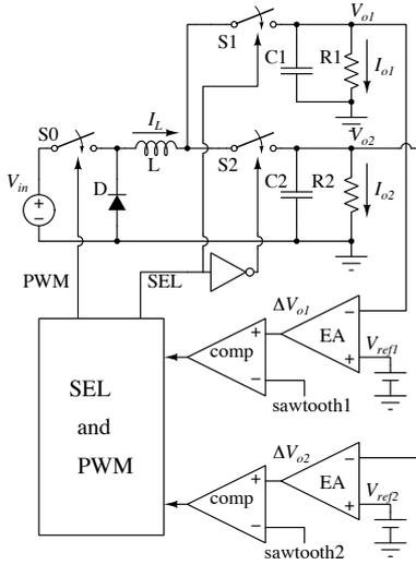
Fig. 4. Schematic diagram of the circuit configuration of the basic buck-buck SIDO converter
