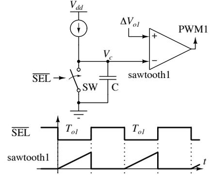
Fig. 10. The basic sawtooth wave generator circuit
