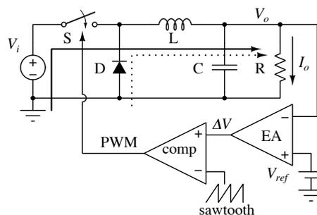
Fig. 1. Schematic diagram of the circuit configuration of the basic buck converter
