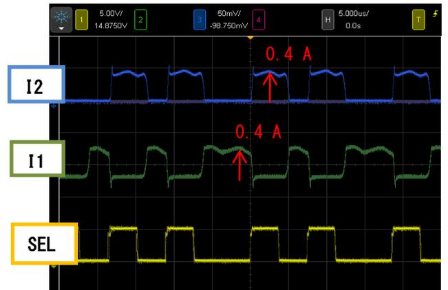
Fig. 19 Experimental signals of SIDO converter
