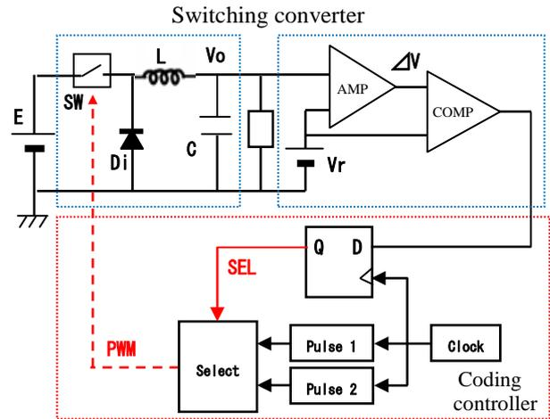
Figure 11. Switching converter with PWM coding.
