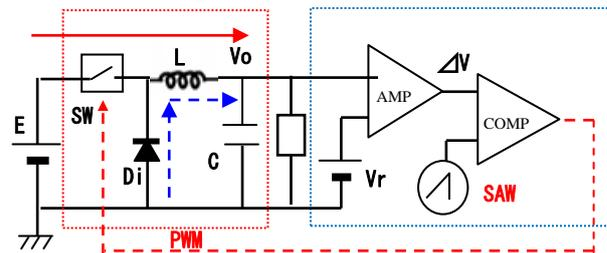
Figure 1. Block diagram of a buck converter.
