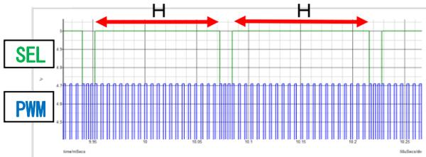
Figure 15. Waveforms of SEL and PWM signals.
