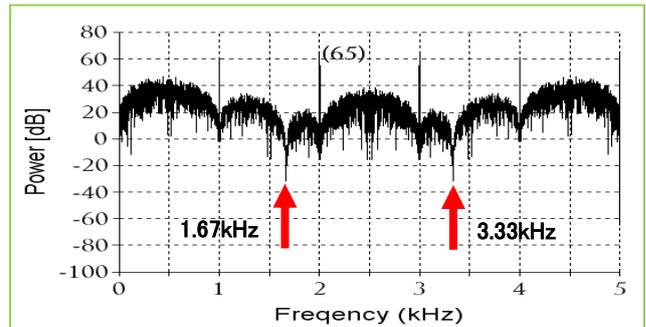
Figure 7. Spectrum of output pulses in PWM (2)
