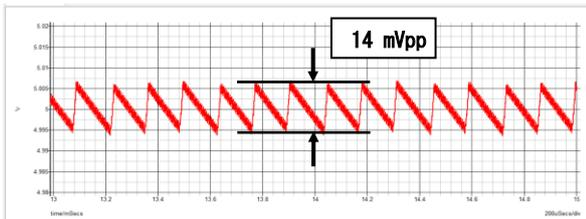
Figure 16. Simulated output voltage ripple of the switching converter with PCM coding.
