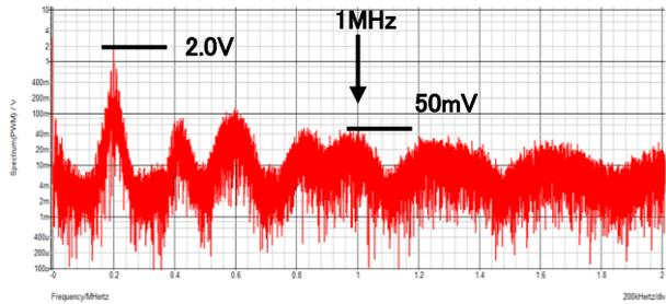
Figure 4. Simulated spread spectrum of the PWM pulse of the buck converter with pulse modulation.
