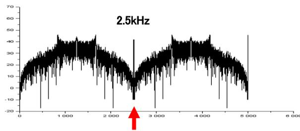
Figure 10. Spectrum of output pulses in PCM (2).
