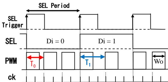
Figure 14. Refined pulse coding with PCM.
