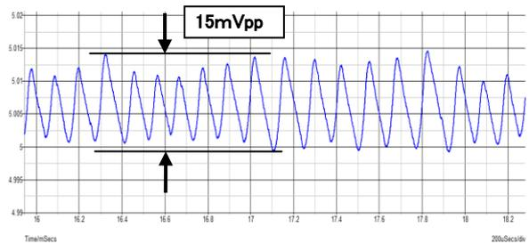
Figure 12. Simulated output voltage ripple of the switching converter with PWM coding.
