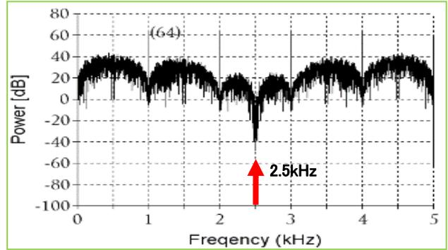
Figure 6. Spectrum of output pulses in PWM (1)
