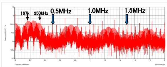
Figure 17. Simulated output voltage spectrum of the switching converter with PCM coding.
