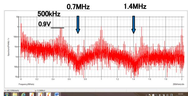
Figure 13. Simulated output voltage spectrum of the switching converter with PWM coding.
