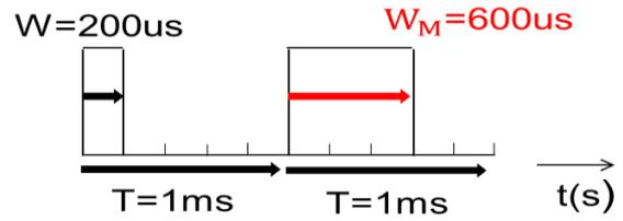
Figure 5. Pulse coding with PWM
