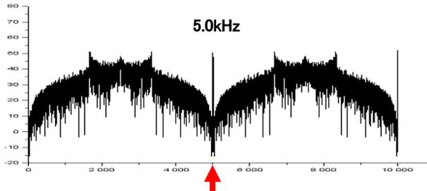
Figure 9. Spectrum of output pulses in PCM (1).
