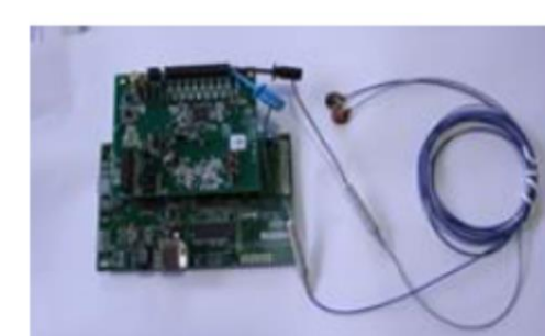
Prototype transmission device (with EEG sensor probe)
