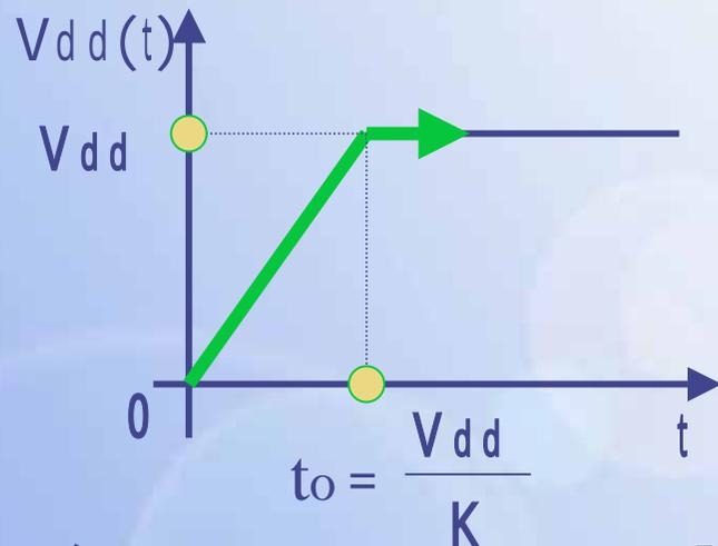
$$\begin{cases} V_{dd}(t) = k \cdot t & (0 \leq t \leq \frac{V_{dd}}{k}) \\ V_{dd}(t) = V_{dd} & (\frac{V_{dd}}{k} \leq t) \end{cases}$$
