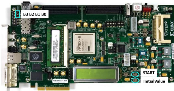
Fig. 9. FPGA Implementation of 4-bit Gray code TDC.
