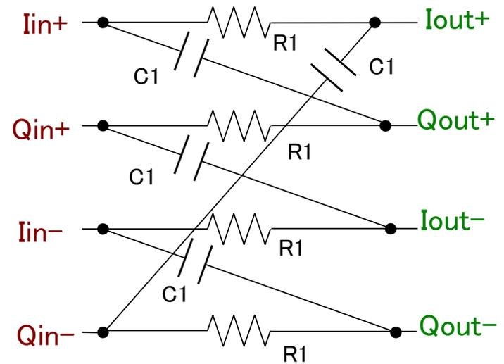
$$R_1 = 1k\Omega \quad C_1 = 10pF$$
