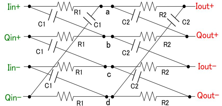
$$R_1 = 1k\Omega \quad C_1 = 10pF$$
