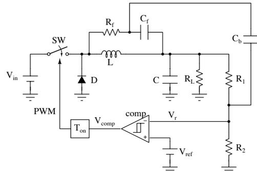
Fig. 1. Buck converter with COT control.
