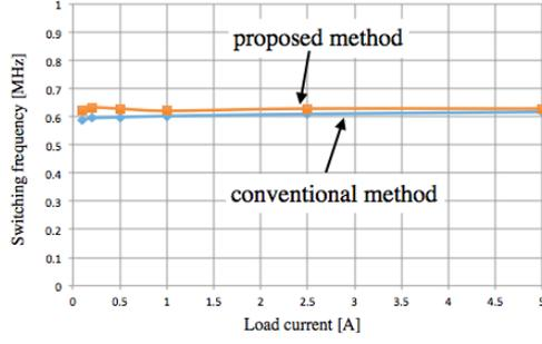
Fig. 8. Switching frequency for output current change.
