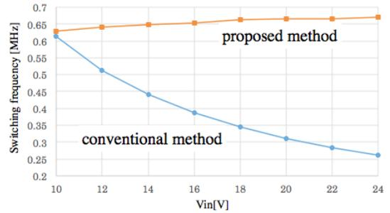
Fig. 6. Switching frequency and input voltage
