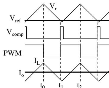
Fig. 2. Waveforms during COT operation.
