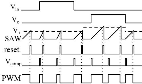
Fig. 4. PWM in response to the input/output voltage change
