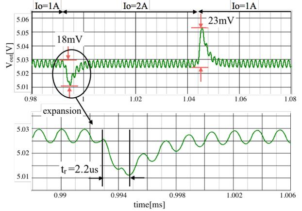
Fig. 5. Simulated output voltage for the load change
