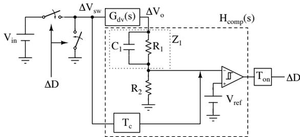
Fig. 9. Block diagram of the proposed circuit in Fig. 3[1]
