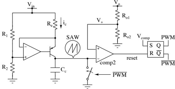
Fig. 3. Proposed  $T_{on}$  pulse generator
