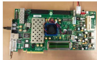
Fig. 12. FPGA board (Xilinx Virtex-6 ML605).
