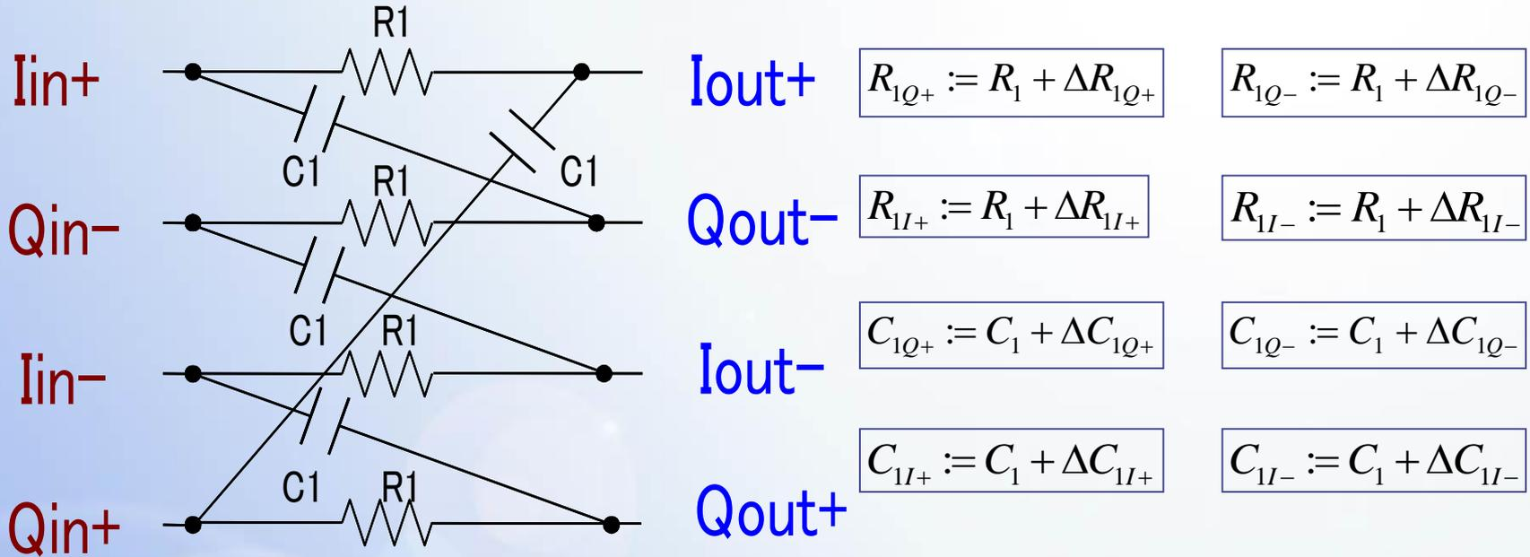
$\Delta R_{1Q+}, \Delta R_{1Q-}, \Delta R_{1I+}, \Delta R_{1I-}$  : 抵抗のばらつき
