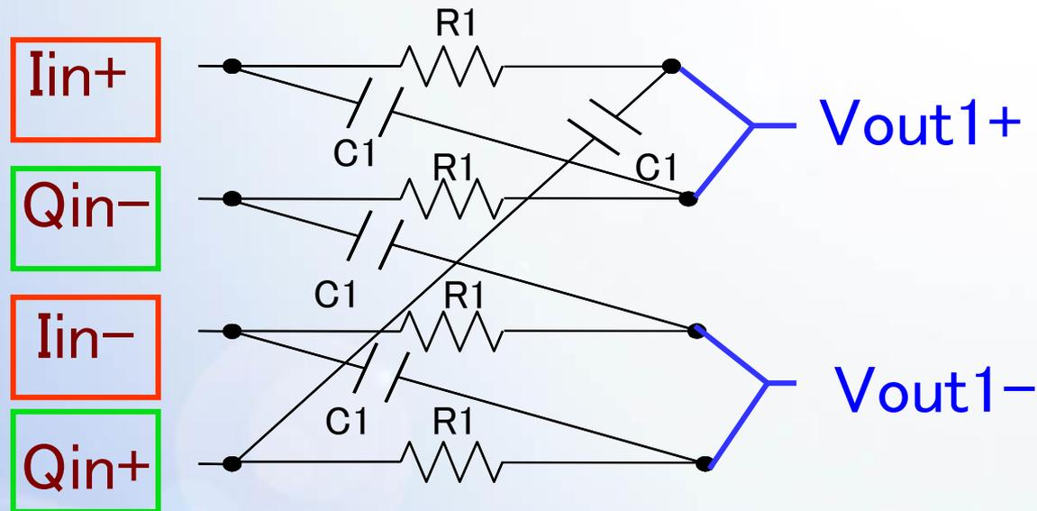
$$V_{out1}(j\omega) = \frac{1}{2} I_{in}(j\omega) - \frac{1}{2} \frac{1 - j\omega R_1 C_1}{1 + j\omega R_1 C_1} Q_{in}(j\omega)$$
