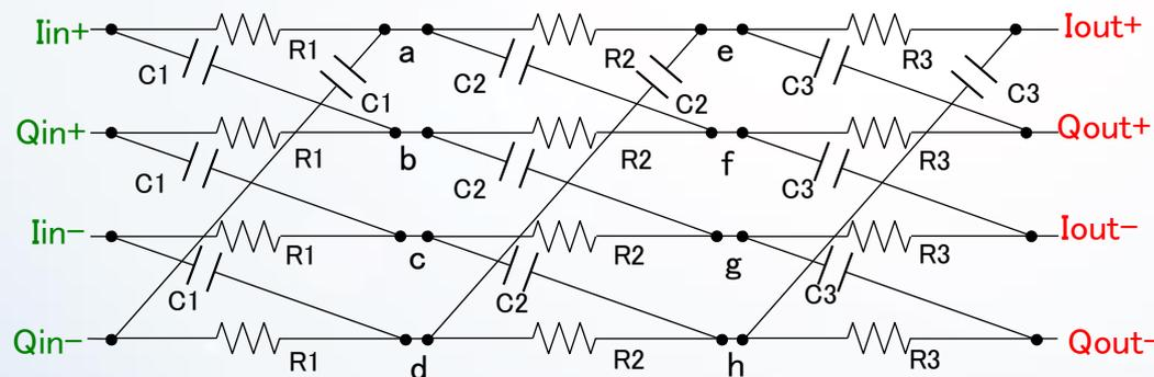
$$N_3(j\omega) = (1 + \omega R_1 C_1)(1 + \omega R_2 C_2)(1 + \omega R_3 C_3)$$
