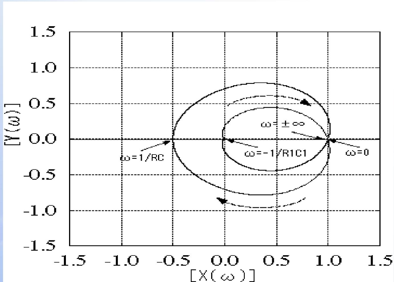
$\cdot RC_1 = R_2C_2 = R_3C_3 = R_4C_4$      $\cdot Y = 0$ で対称
