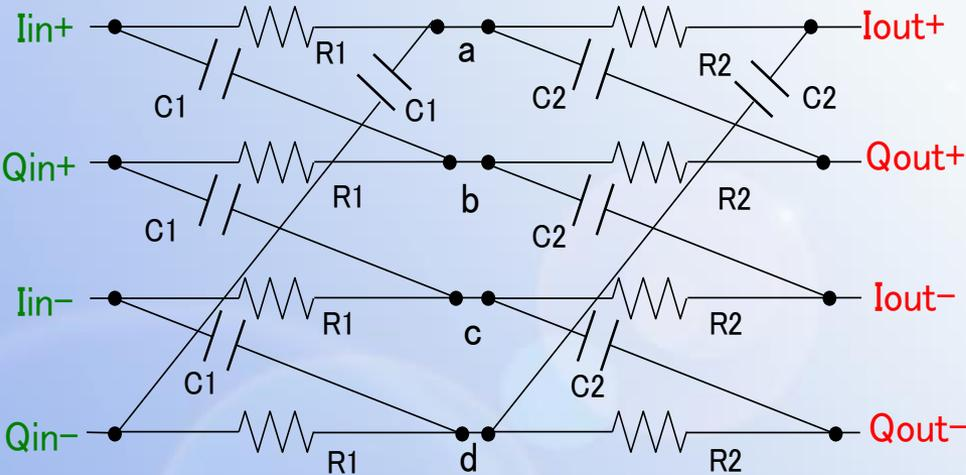
$\omega = -\frac{1}{R_1 C_1}, -\frac{1}{R_2 C_2}$  のゼロ点を持つ
