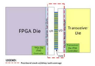
This test methodology is proven reliable with the simulation results showing that various defects can be detected and diagnosed effectively using the proposed methods. Besides, the boundary scan cell proposed here utilizes only half of the registers required by the standard boundary scan cells thus reduces the die area by 50%.
