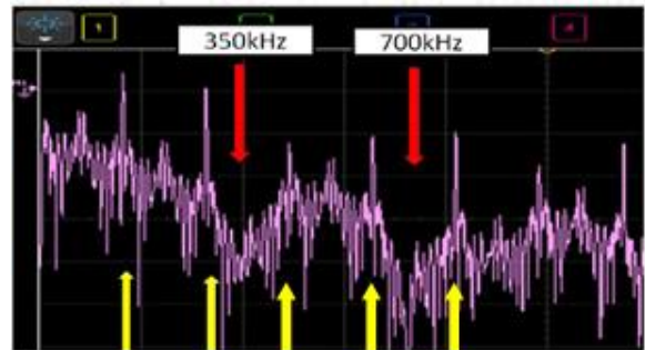
Fig.9 Experimental spectrum of PWC converter 2
