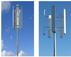
Vertical-axis wind turbines (VAWTs) have the main rotor shaft arranged vertically against wind. It can accept wind from any direction for the operation.
