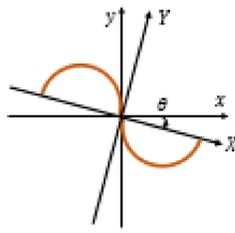
$(X, Y, Z)$ : Position component in rotational coordinate system
