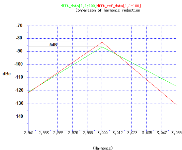
Figure 109 - Comparison of 3 rd harmonic when both 3 rd and 5 th harmonics are suppressed for AWG.
