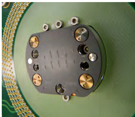
Figure 175 – 16-site EEPROM wafer sort probe head
