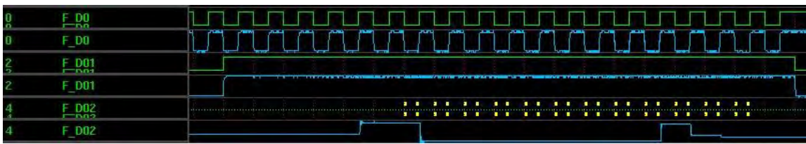
Figure 7 –ams AG SAR ADC DFT clocking and data acquisition scheme
