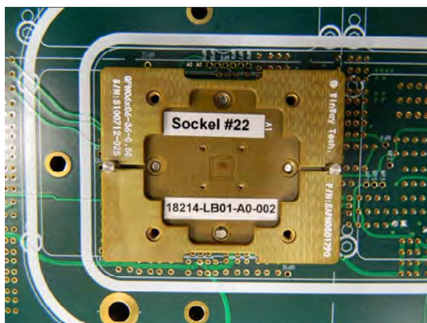
Figure 5 –Winway production socket
