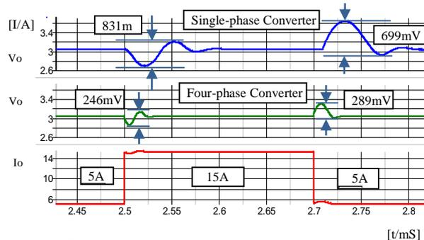
Fig. 6 Comparison of the output voltage ripples. Fig. 7 Comparison of the load fluctuations.
