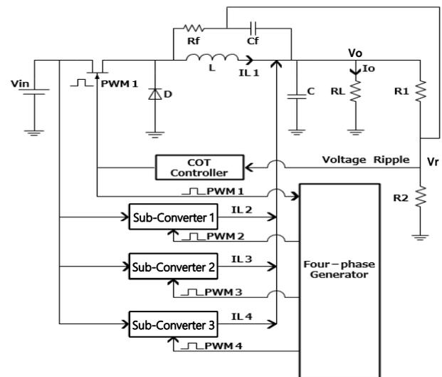
Fig.2 Four-phase converter with COT control
