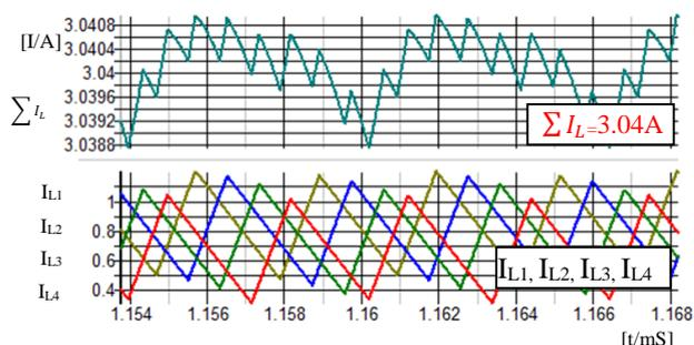
Fig. 5 Simulated waveforms of four-phase converter.
