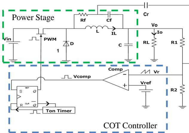
Fig.1 Buck converter with COT control
