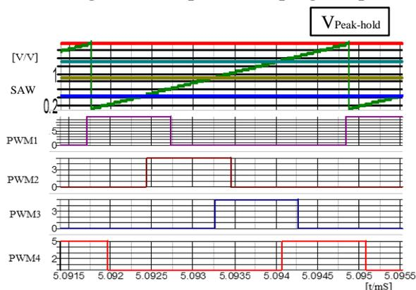
Fig. 4 Simulation result of four-phase PWMs.
