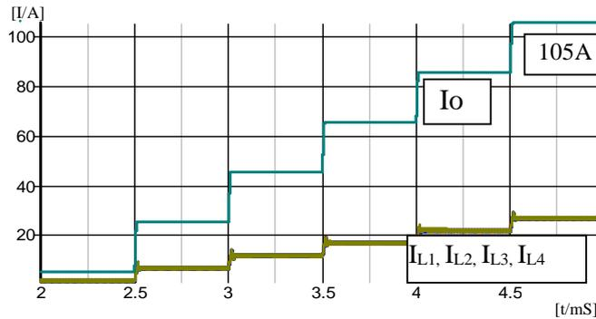
Fig. 8 Simulation result for large load current.
