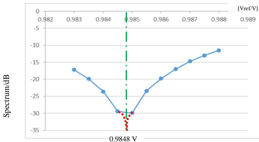
Fig. 12 Relationship between  $V_{ref}$  of COT pulse and converter output spectrum level of conductive noise at  $F_{pwm}$
