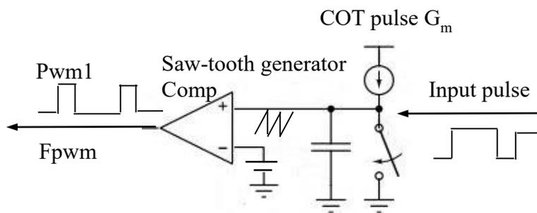
Fig. 9 Proposed COT phase modulation circuit.
