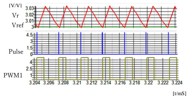
Fig. 3 Simulated waveforms in steady state.
