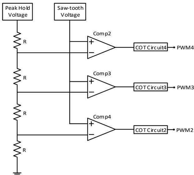
Fig.8 Four-phase pulse generator
