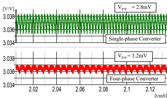
Fig.12 Comparison of the output voltage ripples
