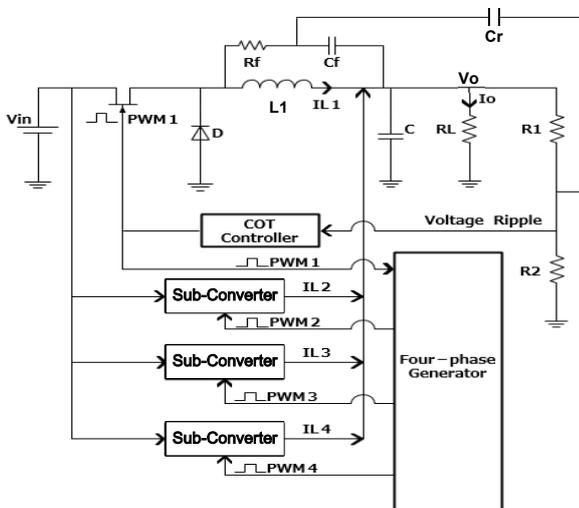
Fig.4 Four-phase converter with COT control
