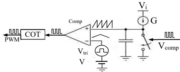
Fig.17 Proposed pulse phase modulation circuit
