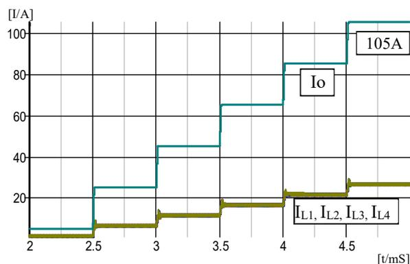
Fig.11 Simulation result of the large load current
