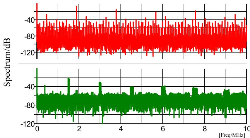
Fig. 20 Up: Without EMI Reduction      Down: With EMI Reduction
