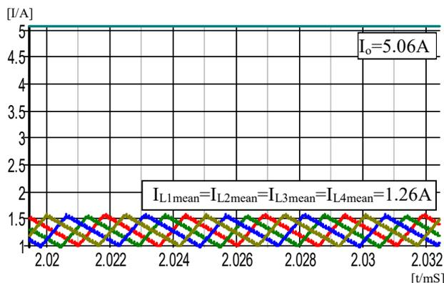
Fig.10 Currents of each phase in the four-phase converter
