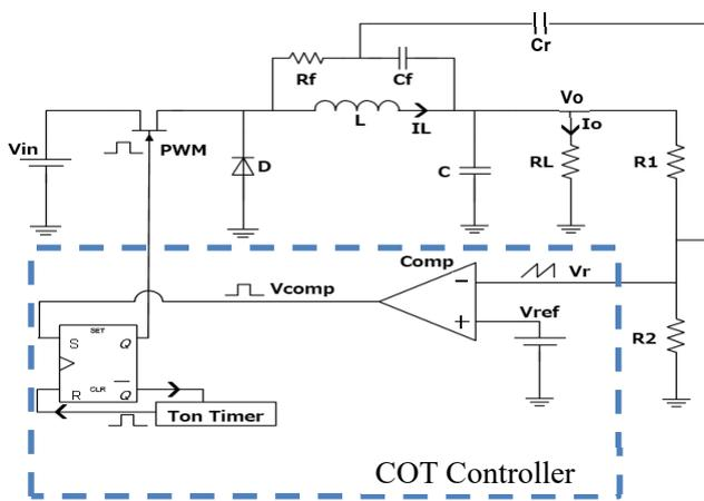
Fig.1 Buck converter with COT control
