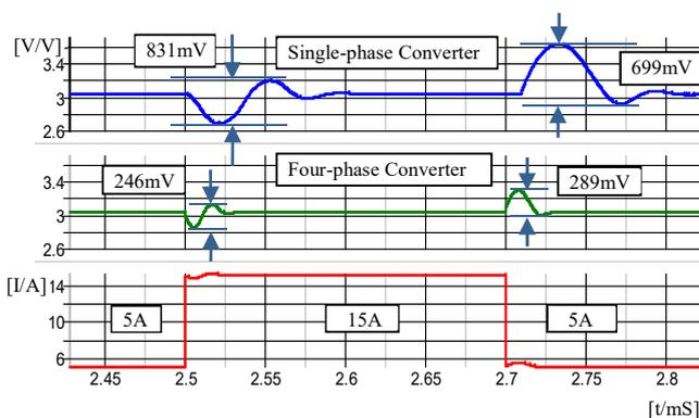
Fig.13 Comparison of the load fluctuations
