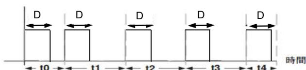
Fig.15 Pulse frequency modulation
