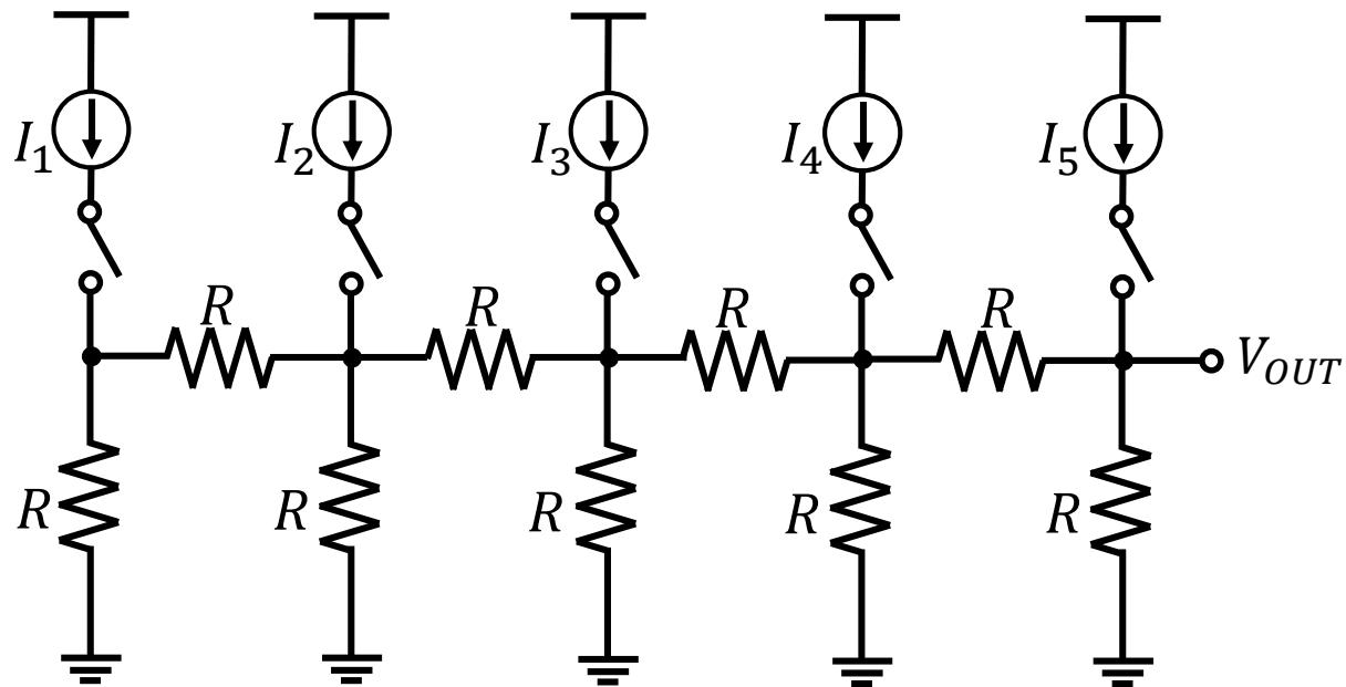
$$V_{OUT}(I_1, I_2, I_3, I_4, I_5, R)$$
