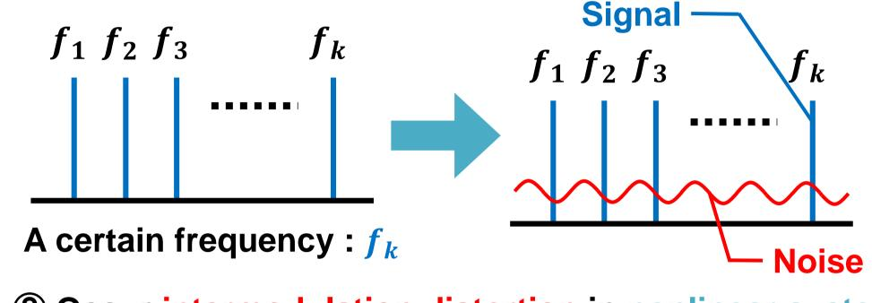
2 Occur intermodulation distortion in nonlinear system
