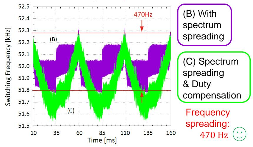
Simulation Result: Spectrum Spreading & Duty Compensation ( $V_{out}$ )
