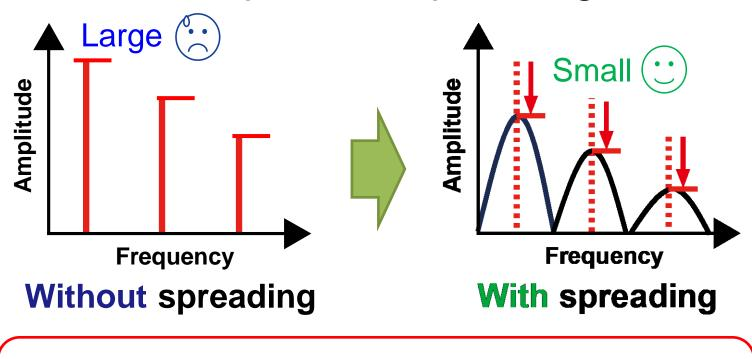
Modulating switching frequency Noise spectrum peak
