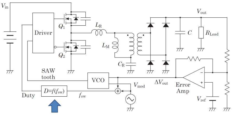
Duty ratio compensation formula  $D = 0.355 \times 10^{-6} f_{sw}^2 - 31.85 \times 10^{-3} f_{sw} + 722.57$  [%]
