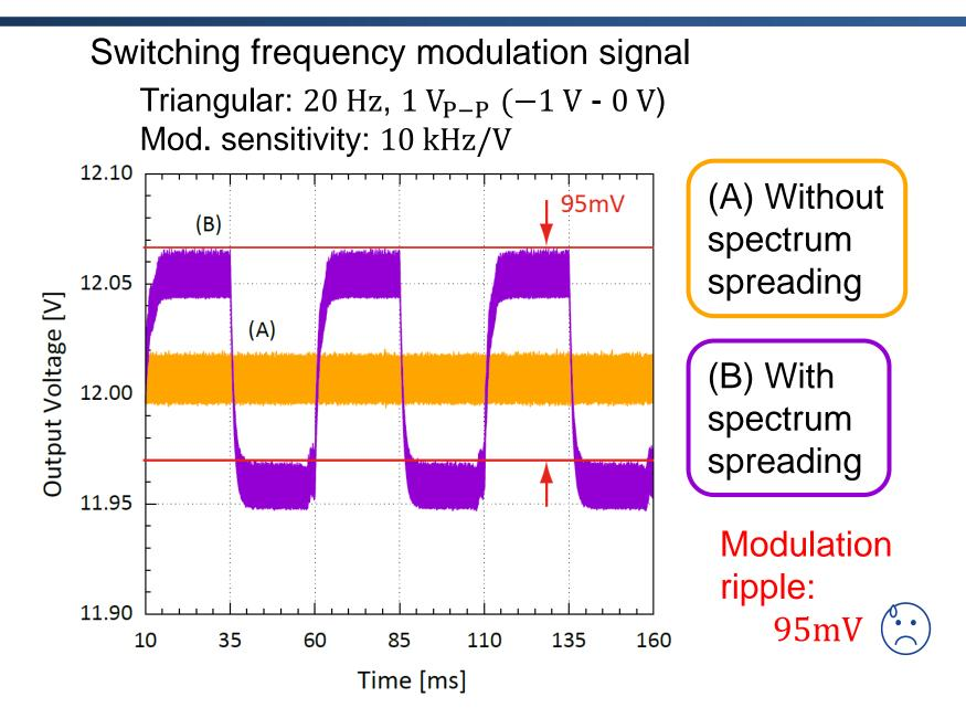
Simulation Result: Spectrum Spreading & Duty Compensation ( $f_{sw}$ )
