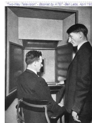
FRANK GRAY and A. L. Johnsrud in television booth. Behind the glass panels at sides and top are the photo-electric cells.
