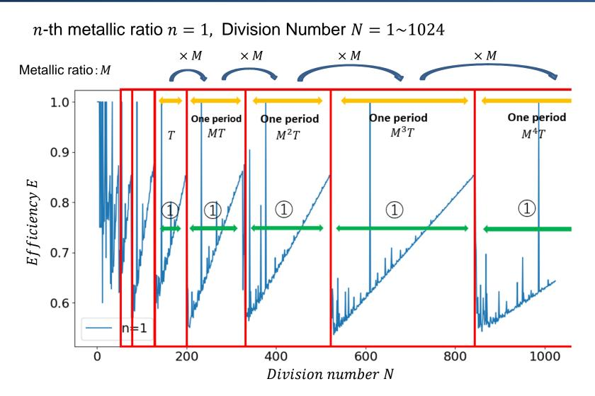
If one period is sawtooth wave, similar waveform is repeated. Cycle length is multiplied by golden ratio for each cycle. 22/33
