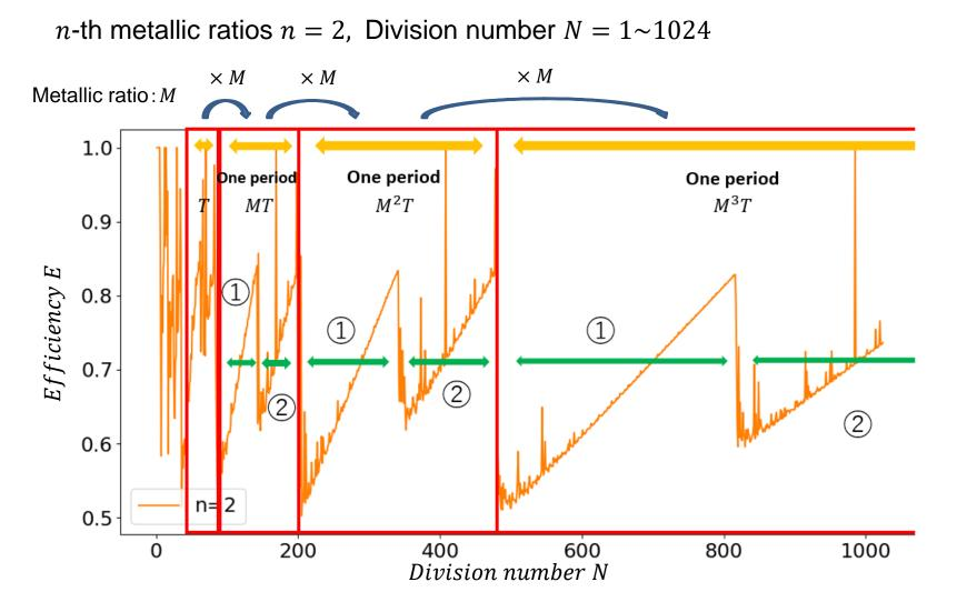
If one period is two sawtooth waves, similar waveform is repeated. Cycle length is multiplied by silver ratio for each cycle.
