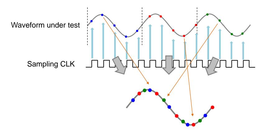
Sampling repetitive waveform with asynchronous CLK Construct one-period waveform
