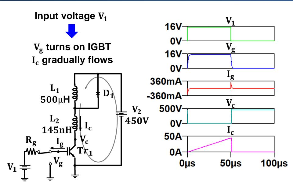
Voltage-Driven IGBT Evaluation Circuit (2/2)
