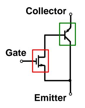
Input part is **MOSFET** Output part is bipolar transistor
