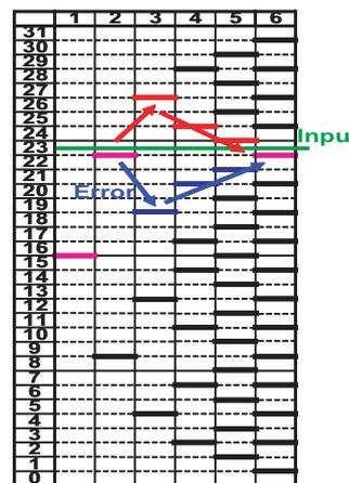
Fig. 5. Operation of the redundant search algorithm of a 5-bit SAR ADC with 6 steps (case 2).
