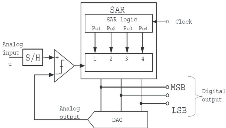
Fig. 1. Block diagram of an SAR ADC.
