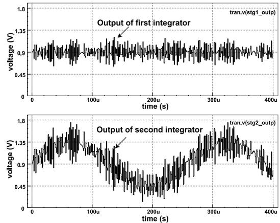
Fig. 8 SPICE simulation results of two-integrator outputs in the proposed  $\Delta\Sigma$ AD modulator.
