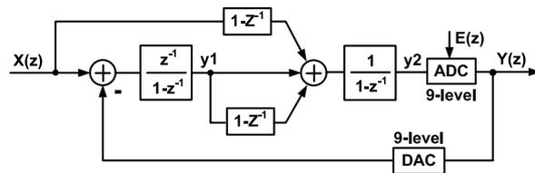
Fig. 3 Proposed second-order feedforward  $\Delta\Sigma$ AD modulator.
