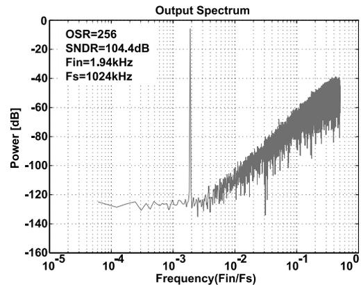
Fig. 5 Simulated output power spectrum of the conventional second-order feedforward  $\Delta\Sigma$ AD modulator in Fig. 2 with harmonic distortions.
