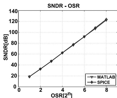
Fig. 10 MATLAB and SPICE simulated SNDR-OSR comparison of the proposed multibit  $\Delta\Sigma$ AD modulator.
