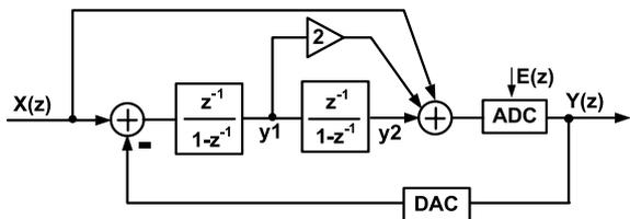
Fig. 2 Conventional second-order feedforward  $\Delta\Sigma$ AD modulator.
