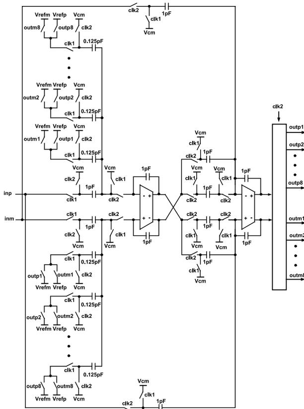
Fig. 7 Switched-capacitor implementation of the proposed feedforward  $\Delta\Sigma$ AD modulator.
