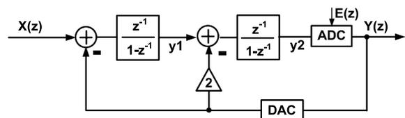
Fig. 1 Second-order feedback  $\Delta\Sigma$ AD modulator.
