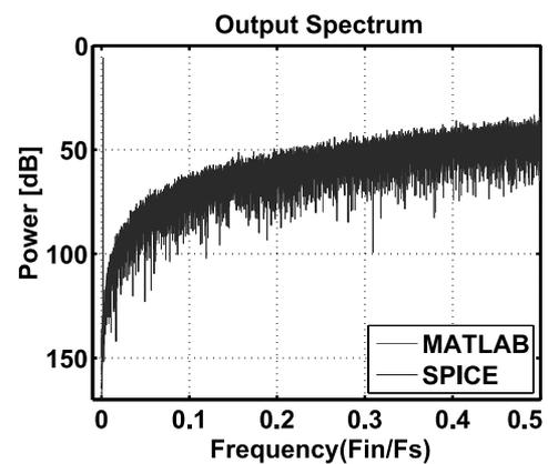
Fig. 9 MATLAB and SPICE simulated output power spectrum comparison of the proposed multibit  $\Delta\Sigma$ AD modulator.
