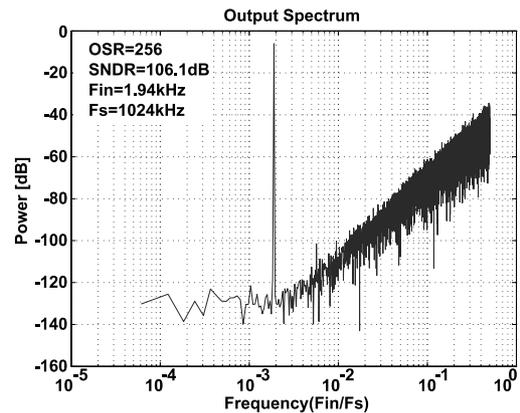
Fig. 6 Simulated output power spectrum of the proposed second-order feedforward  $\Delta\Sigma$ AD modulator in Fig. 3 with harmonic distortions.
