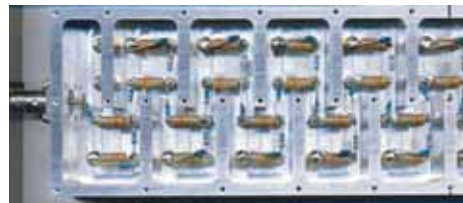
Fig.6: A photo of our BPF. Components are stud-mounted in cavities of a cast-aluminum block. The holes shown are prepared for screw up.
